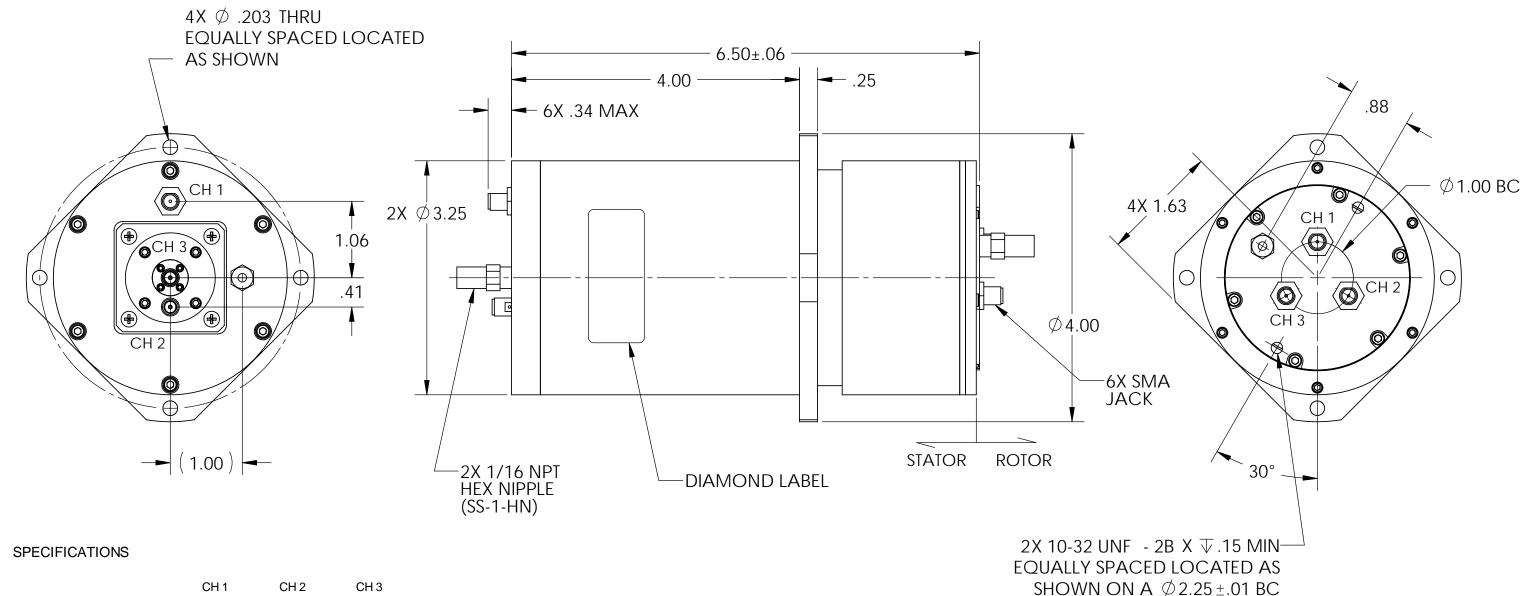
CH 1 CH 2 CH3 Frequency (GHz): 1.435-2.485 1.435-2.485 1.435-2.485 VSWR (max): 1.5:1 1.5:1 1.5:1 Insertion Loss (max): 0.8 dB 0.8 dB 1.0 dB Power (avg): 1W 1W Isolation (min): -40dB--
