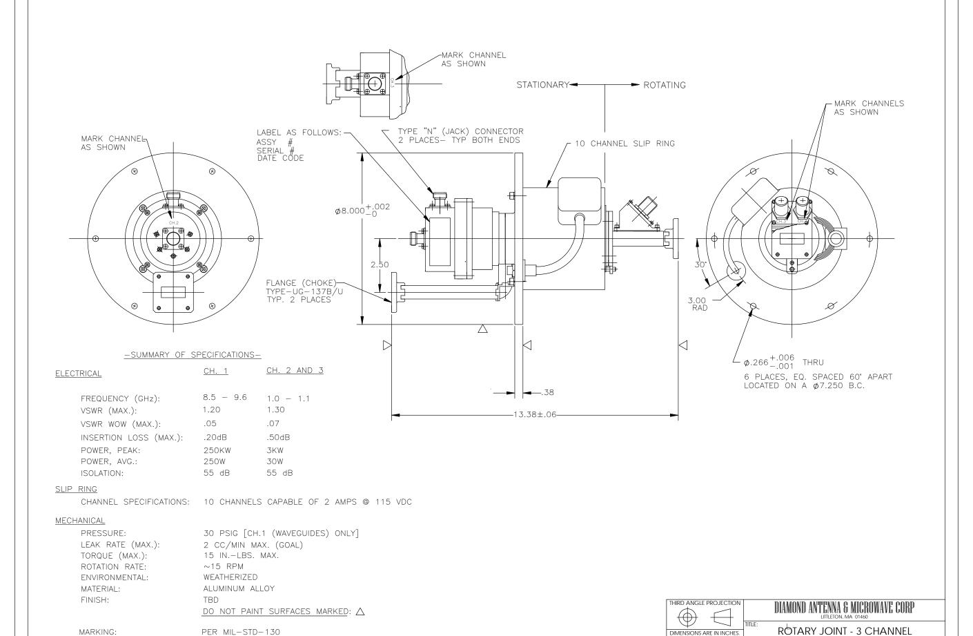
DIMENSIONS ARE IN INCHES. REMOVE ALL BURRS AND SHARP EDGES .005 MAX, UNILESS OTHERWISE SPECIFIED, SURF FINISH 63 TOLERANGES ARE:
