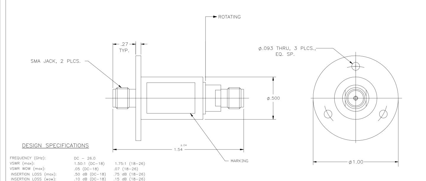
ROTATIONAL SPEED: 50 RPM nom., 500 RPM max. TORQUE: 4 oz.-in. max., 2 oz.-in. nom. OPERATING TEMP: -40° TO +70° C LIFE (min): 5000 HOURS @ 50 RPM
