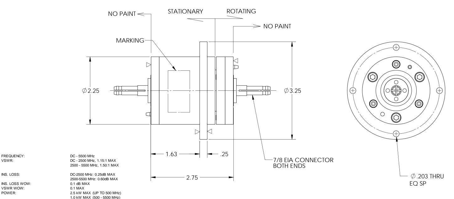
WEATHERIZATION: YES PRESSURIZATION: 30 psig LEAK RATE: 5cc/min. MAX STARTING TORQUE: 60 oz-in, NOM COAX LINE IMPEDANCE: 50 ohms ROTATIONAL SPEED: 100 RPM, MAX MATERIAL: ALUMINUM FINISH: **IRIDITE & TBD PAINT**
