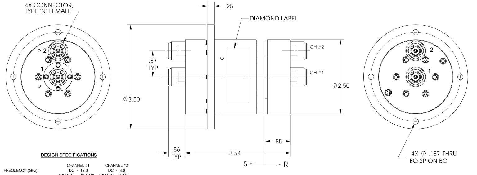
(DC-2.4) (2.4-12) (DC-2.4) (2.4-3) VSWR (MAX): 1.25:1 1.60:1 1.25:1 2.5:1 VSWR WOW (MAX): .05 .10 .05 .10 INSERTION LOSS (MAX): .50 dB .20 dB .50 dB .20 dB I.L. WOW (MAX): .10 dB .10 dB .20 dB POWER, PEAK (MIN): 10 KW 10 KW POWER, AVERAGE (MIN): 200 W (@1 GHz) 200 W (@1 GHz) ISOLATION (MIN): <----- 50 dB -----
