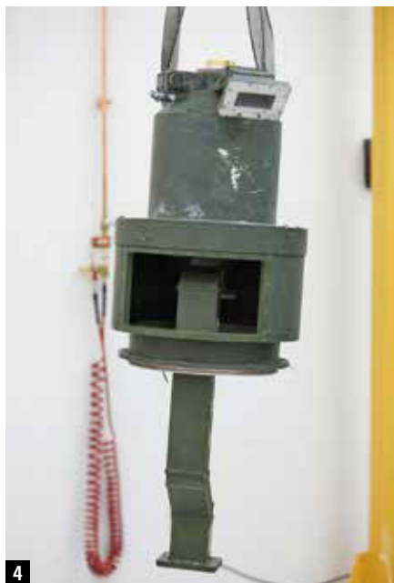
1 Diamond Series 2920 Primary & Secondary ATC Radar Rotary Joint 2 Diamond Series 2355 Secondary Surveillance Radar 3 Diamond technicians reassembling a repaired RF rotary joint 4 A failed RF rotary joint ready for refurbishment 5 Diamond Series 26102 Airport Surveillance Radar
